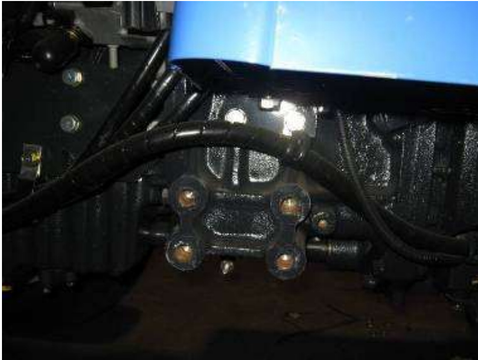
Picture to locate the holes of front coupling.
